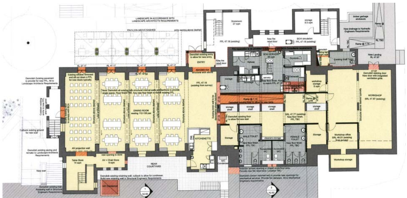
Figure 2.4 Plan showing the footprint of the proposed new buildings in the Village Green Precinct and the building use to be provided by this stage of the project
