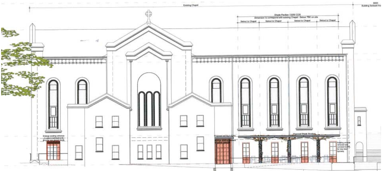
Figure 2.3 Plan showing the proposed minor changes to the north elevation of the Chapel to facilitate the community use of the undercroft
