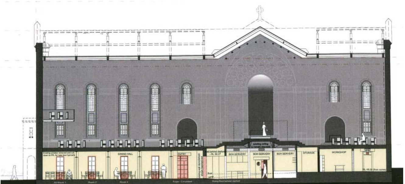
Figure 2.5 Cross section plan showing the proposed changes to the undercroft space
