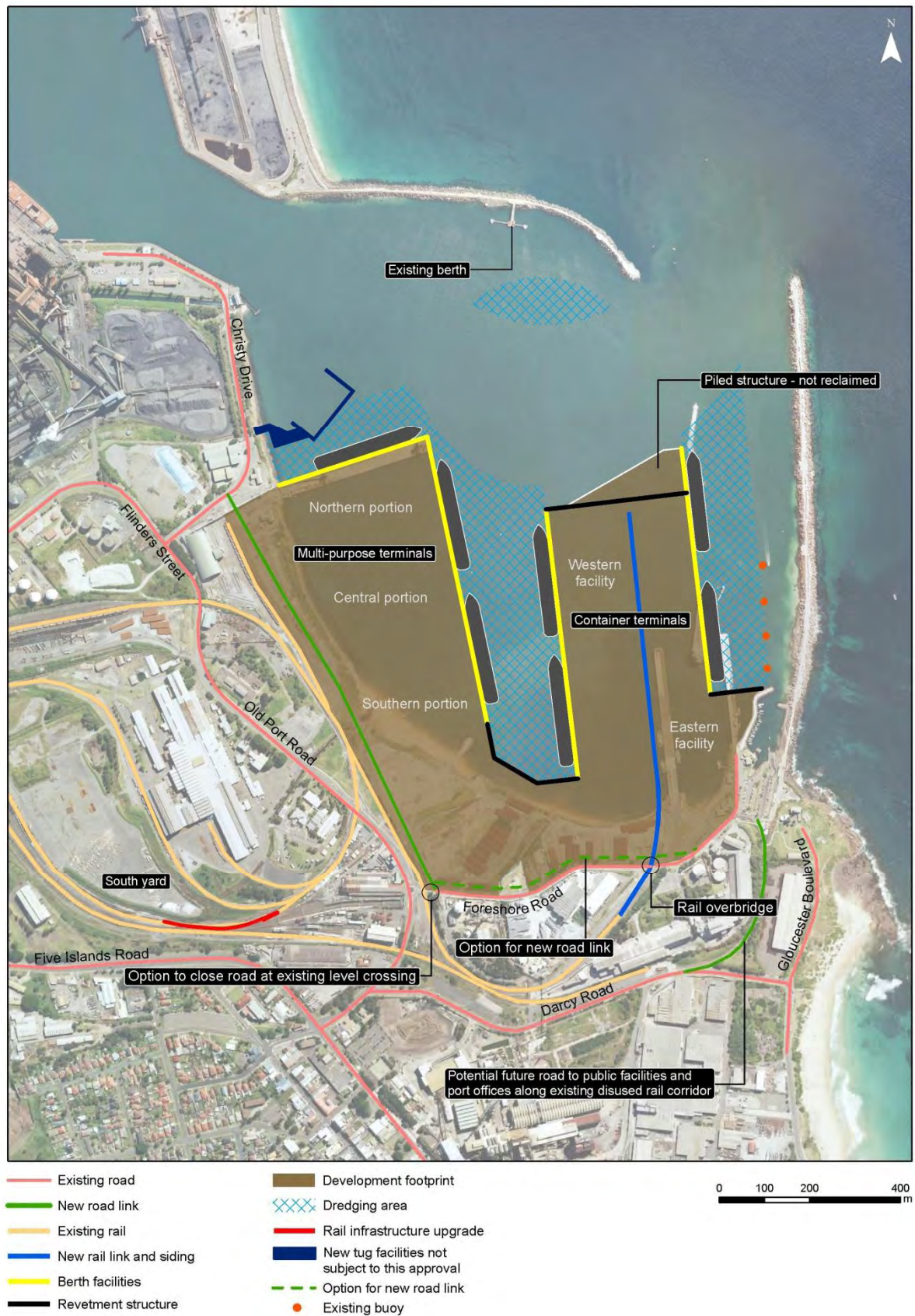
Figure 3.2: PKPC Outer Harbour Development Final Layout
