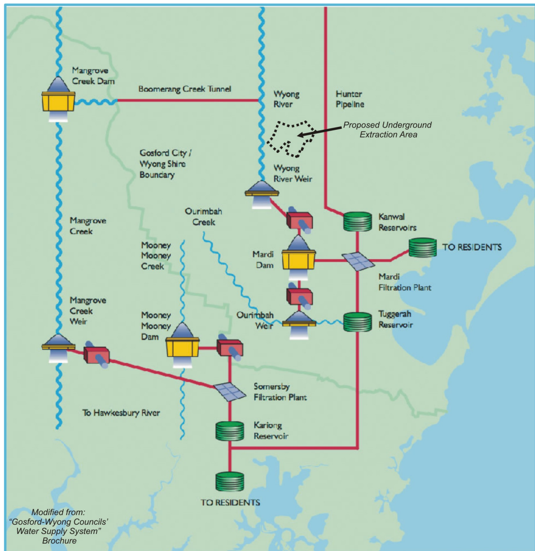
Figure 7.2 Schematic Diagram of Water Supply System and Mine Location
