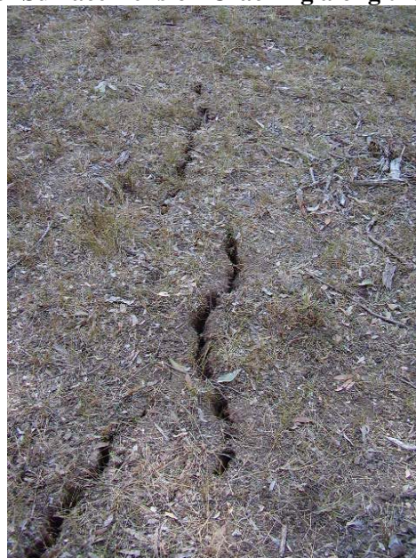
Fig. 4.13 Example of Surface Tension Cracking along the Top of a Steep Slope
