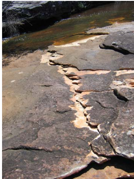
Fig. 4.14 Example of Sandstone Fracturing and Bedding Plane Slippage in Bedrock in the Base of a Stream in the Southern Coalfield (NB: no significant bedrock lined streams occur in W2CP study area)
