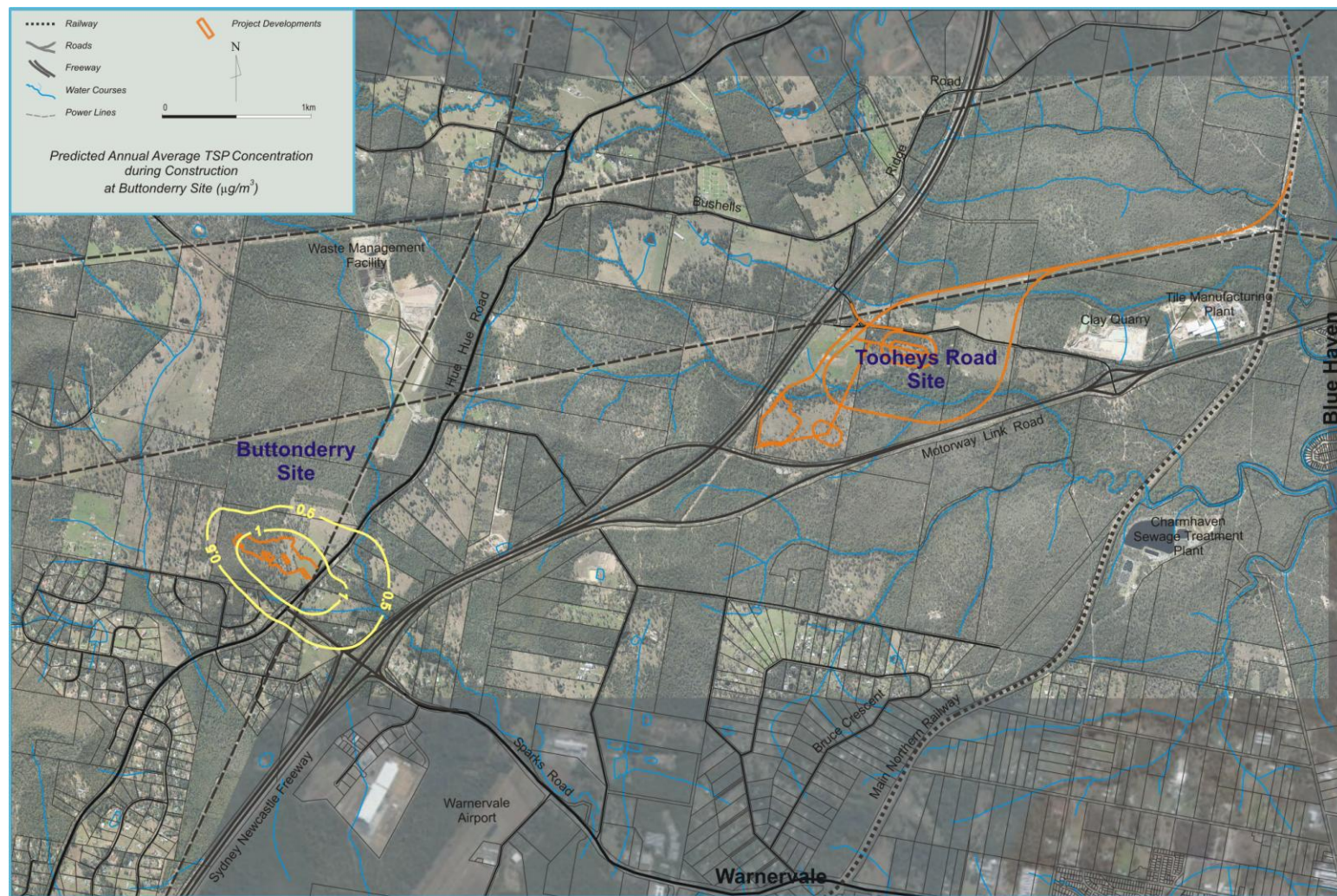
Figure 12 Predicted annual average TSP concentration during construction at the Buttonderry site ( \mu\text{g}/\text{m}^3 )
