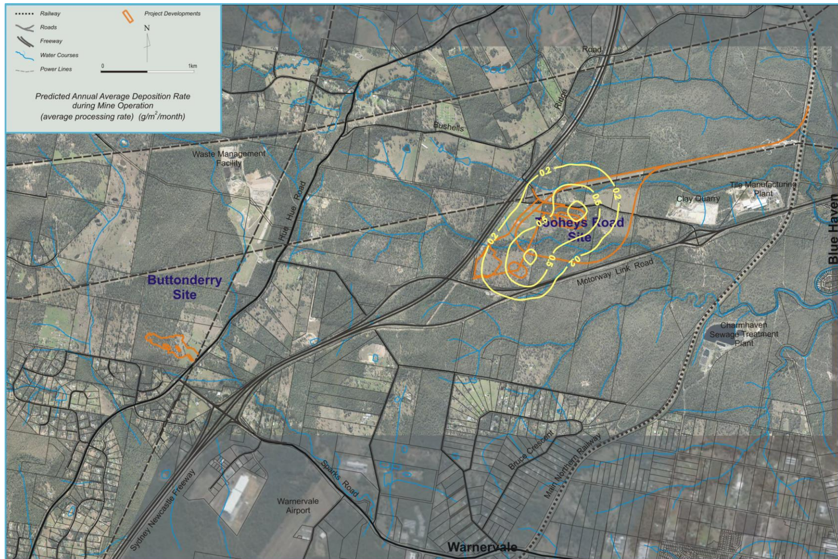
Figure 22 Predicted annual average dust deposition during mine operation (g/m 2 /month)
