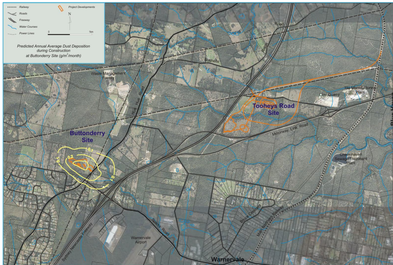
Figure 13 Predicted annual average dust deposition construction at the Buttonderry site ( \text{g/m}^2/\text{month} )
