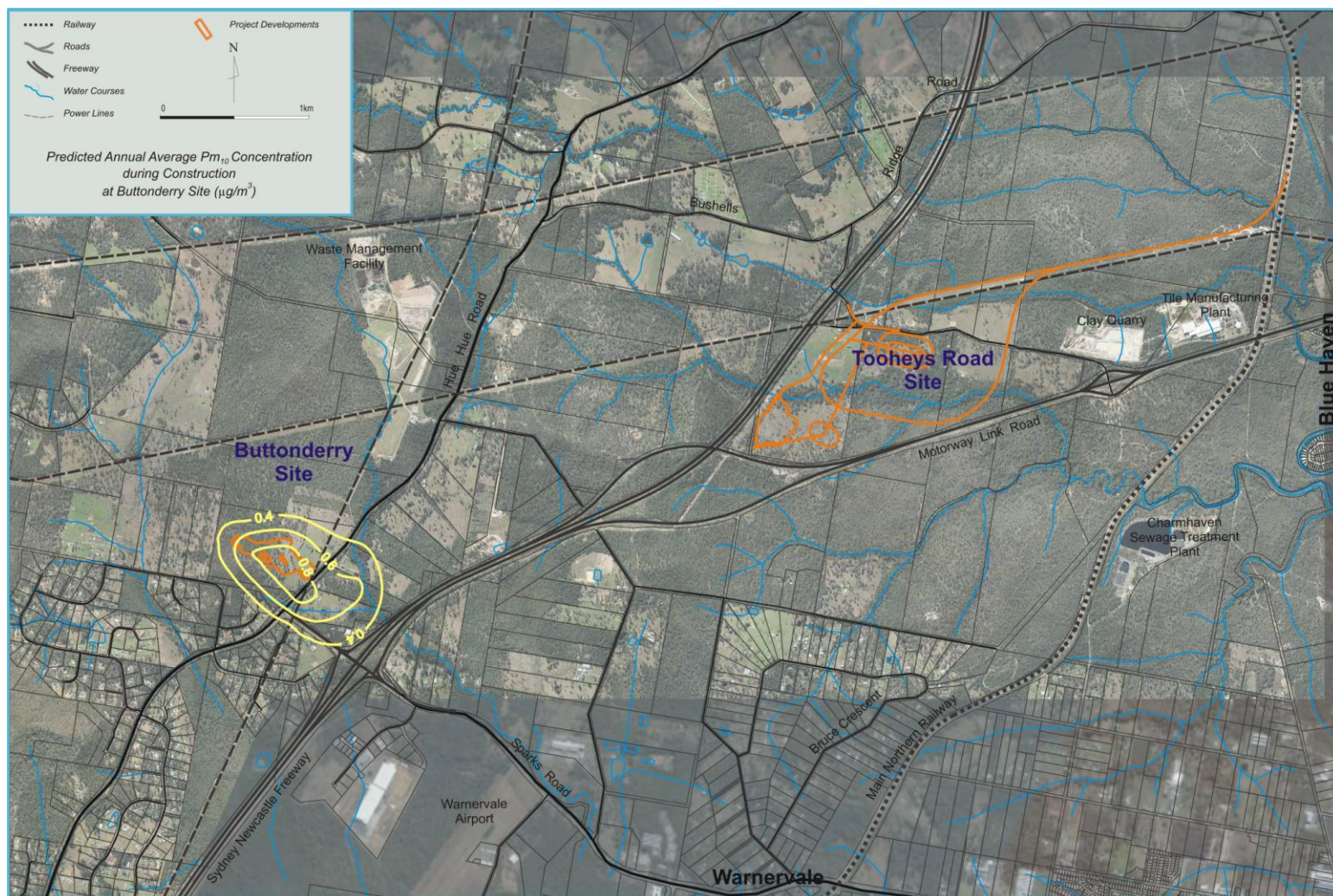
Figure 11 Predicted annual average PM_{10} concentration during construction at the Buttonderry site ( \mu g/m^3 )
