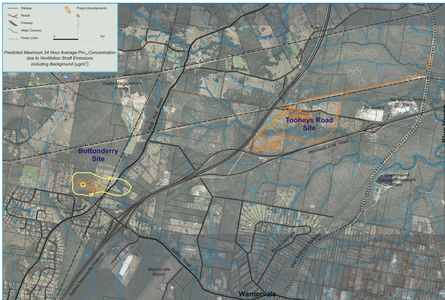
Figure 25 Predicted maximum 24-hour average PM 10 concentration due to ventilation shaft emissions plus background (µg/m 3 )
