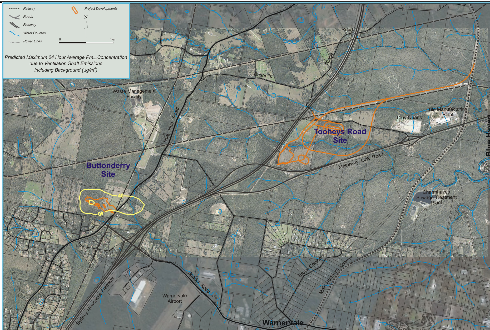
Figure 12.17 Predicted Maximum 24 Hour Average PM_{10} Concentration Due to Ventilation Shaft Emissions, including Background
