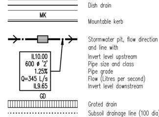
Subsoil drainage line (100 dia) ······ FP Flushing point
