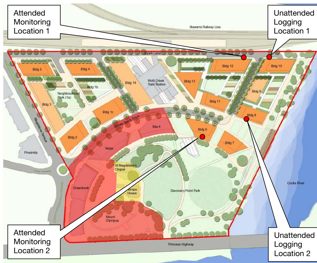
Figure 2 Noise and Vibration Measurement Locations
