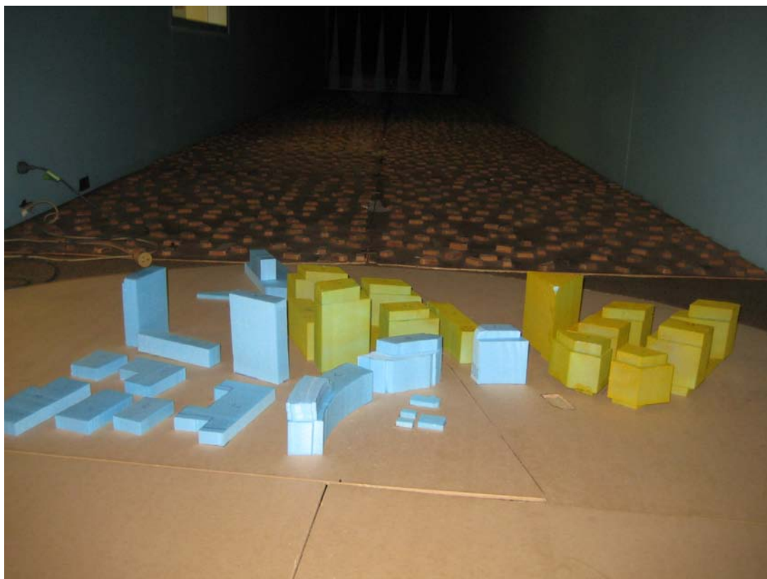
Figure 4 Scaled Development Model in Wind Tunnel (View from East)
