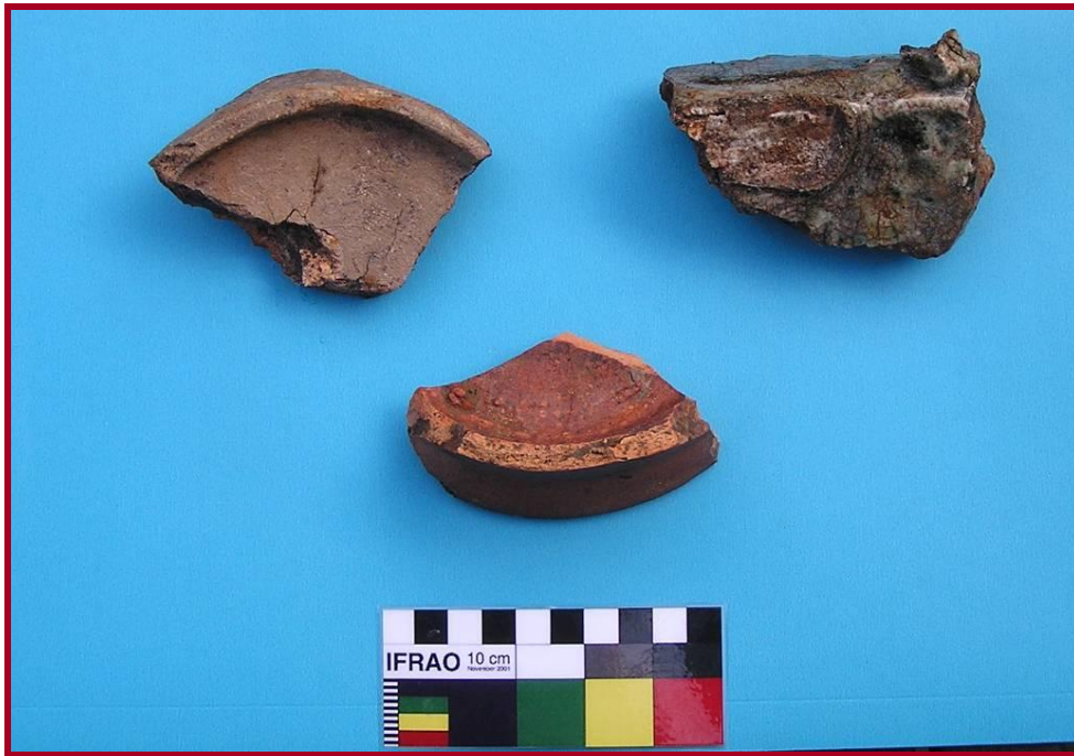
Figure 33. Examples of early pottery wasters probably from Fowler's works. Note the vitrified sagger (kiln furniture) at top right.
