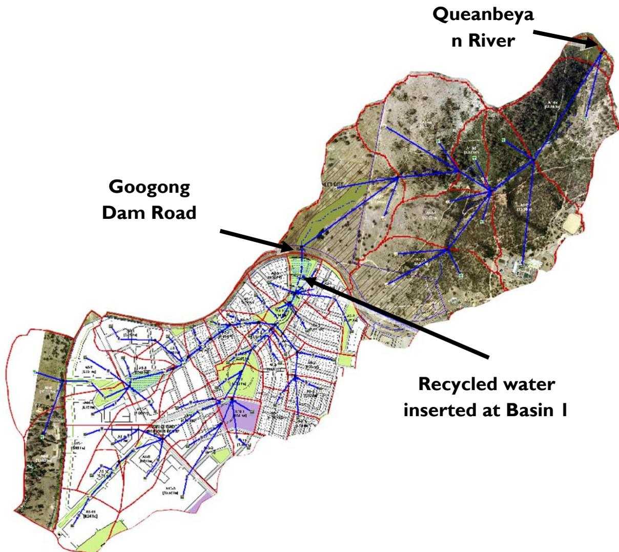
**Figure 14 Developed Catchment MUSIC Model (WSUD Recycled at Basin 1 – Revised Bioretention)**
