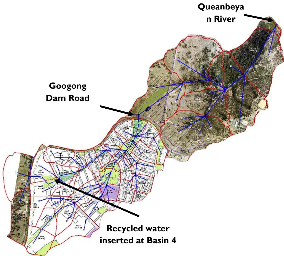
**Figure 16** Developed Catchment *MUSIC* Model (WSUD Recycled at Basin 4 – Revised Bioretention)
