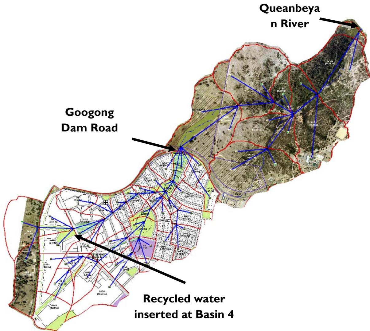
**Figure 17** Developed Catchment *MUSIC* Model (WSUD Recycled at Basin 4 – Revised Bioretention with Rainwater Tanks)
