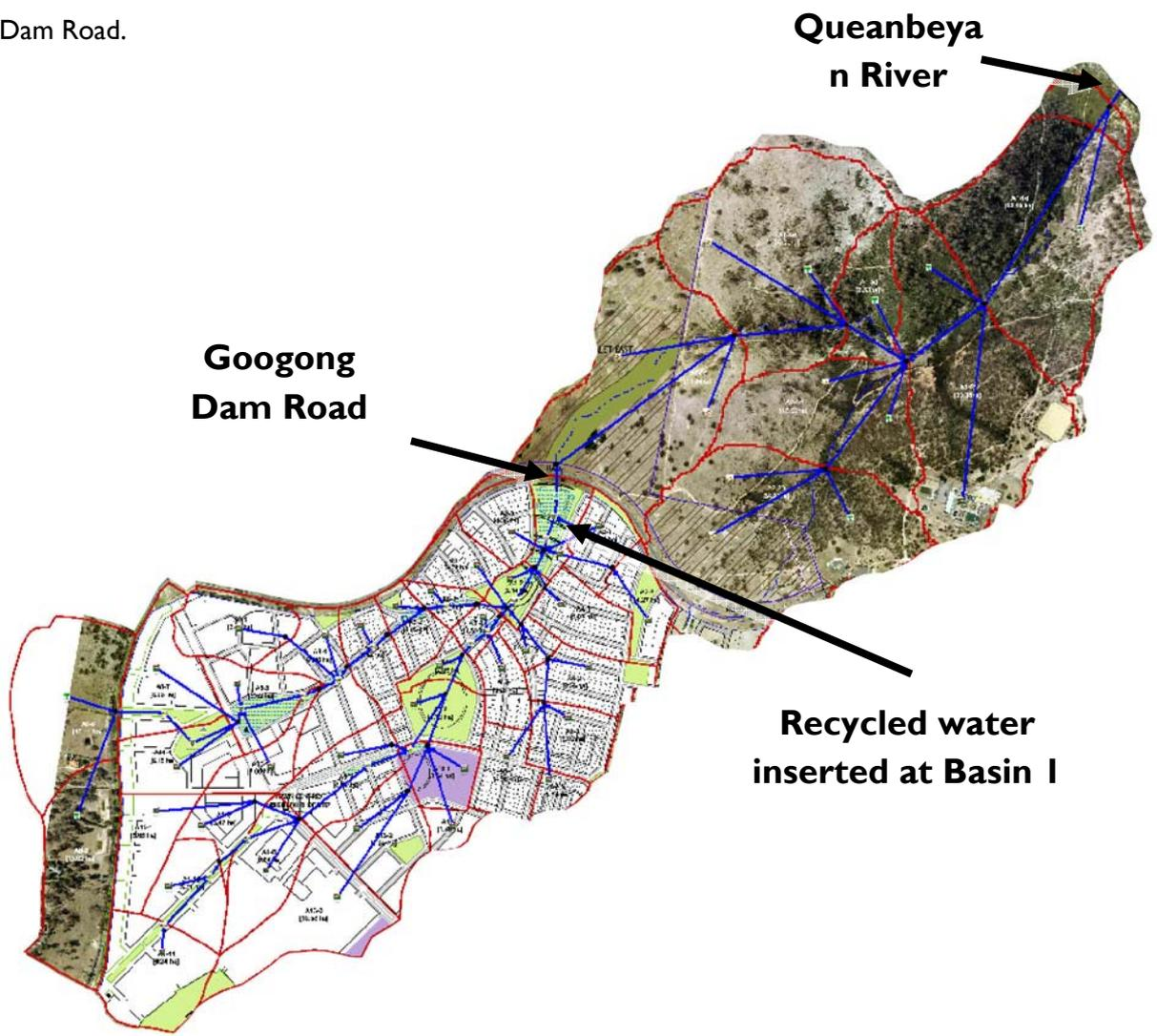
**Figure 13** Developed Catchment *MUSIC* Model (WSUD Recycled at Basin 1)
