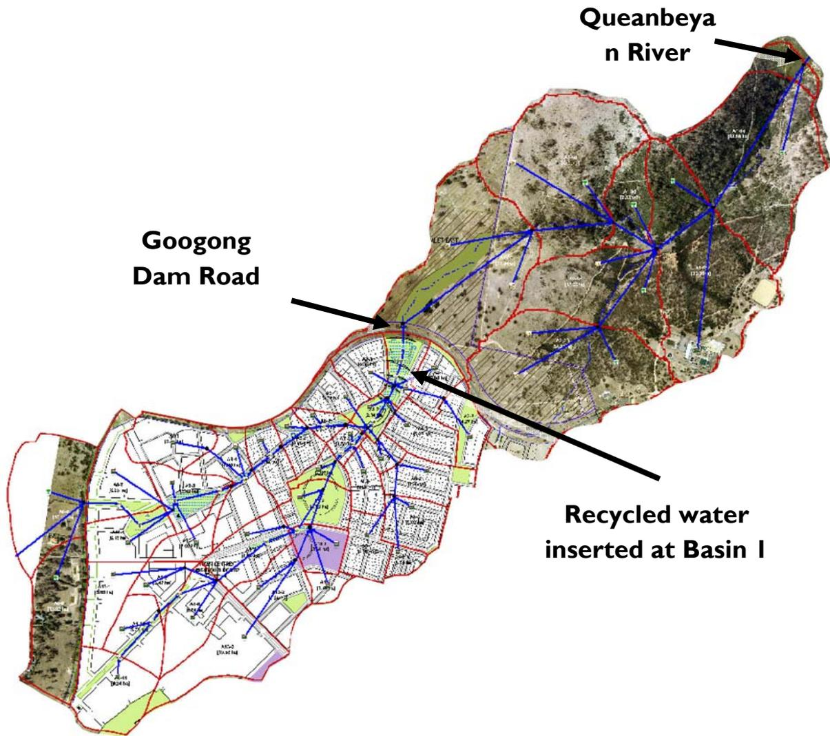
**Figure 15** Developed Catchment *MUSIC* Model (WSUD Recycled at Basin 1 – Revised Bioretention with Rainwater Tanks)
