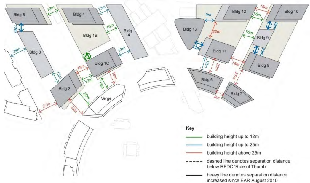
Figure 6 – Building separation of indicative floor layout (PPR)
