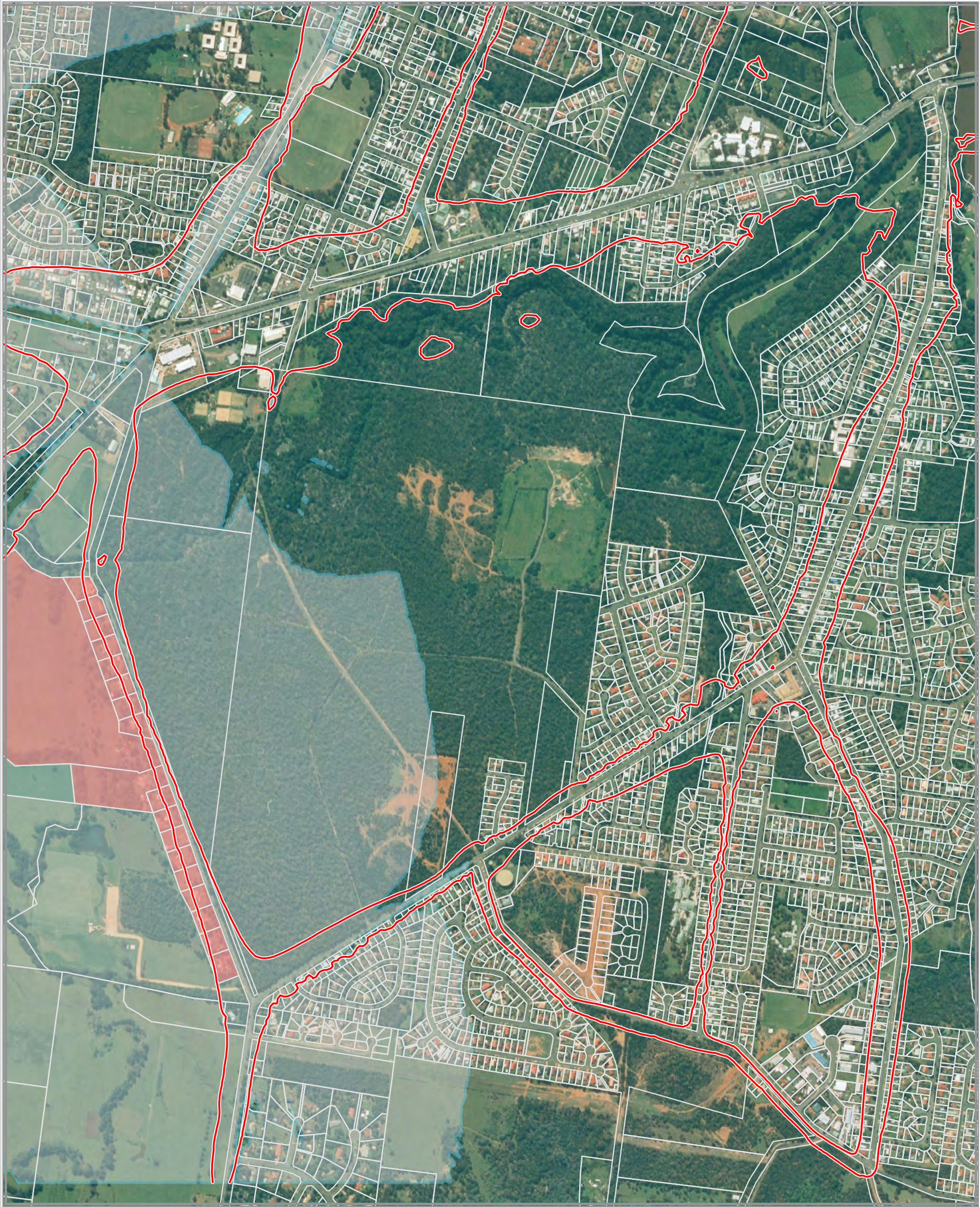
Option 3 Facade noise levels - Impact from new roads (increase of 0.5 dB(A))
