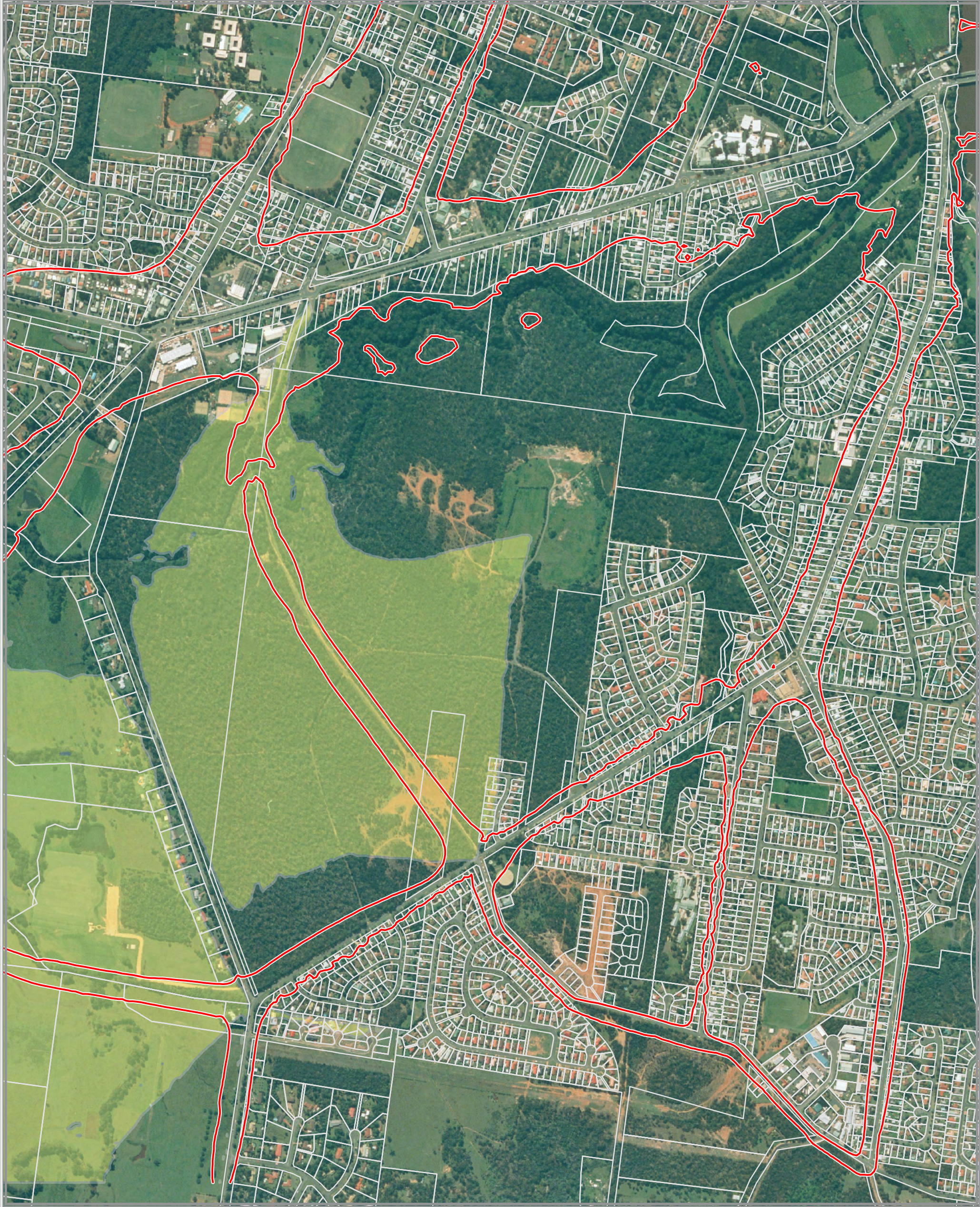
Option 1 MVR Facade noise levels - Impact from existing roads (increase of 2 dB(A))
