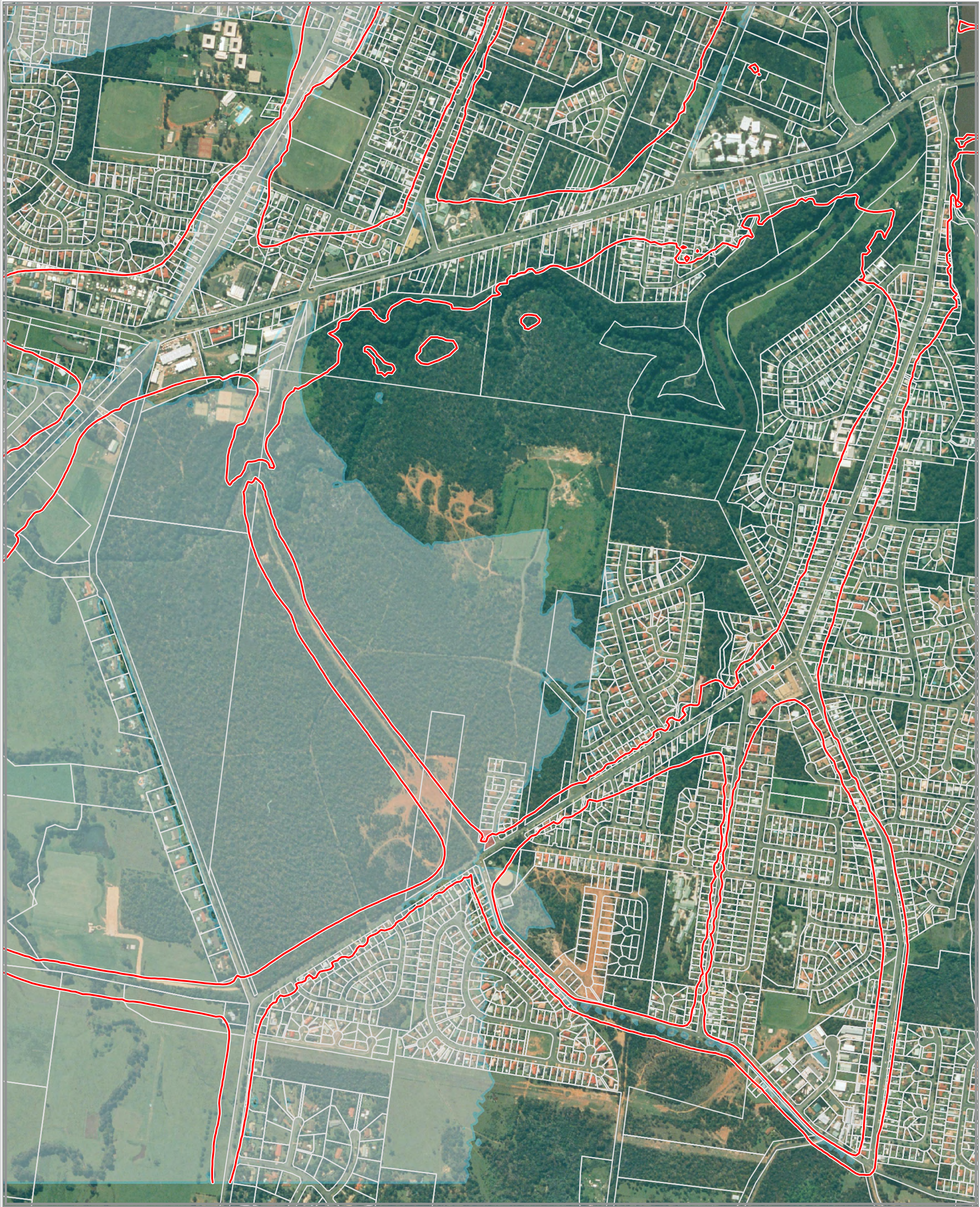
Option 1 MVR Facade noise levels - Impact from new roads (increase of 0.5 dB(A))
