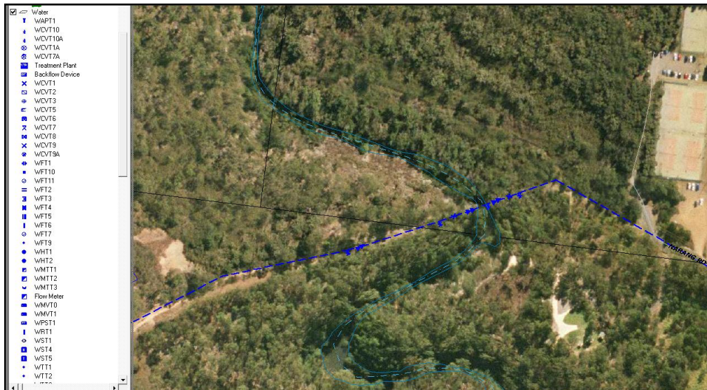
Above: Aerial photograph shows the location of the water trunk main in the sensitive environmental area aside the schematic bridge proposal at the creek crossing
