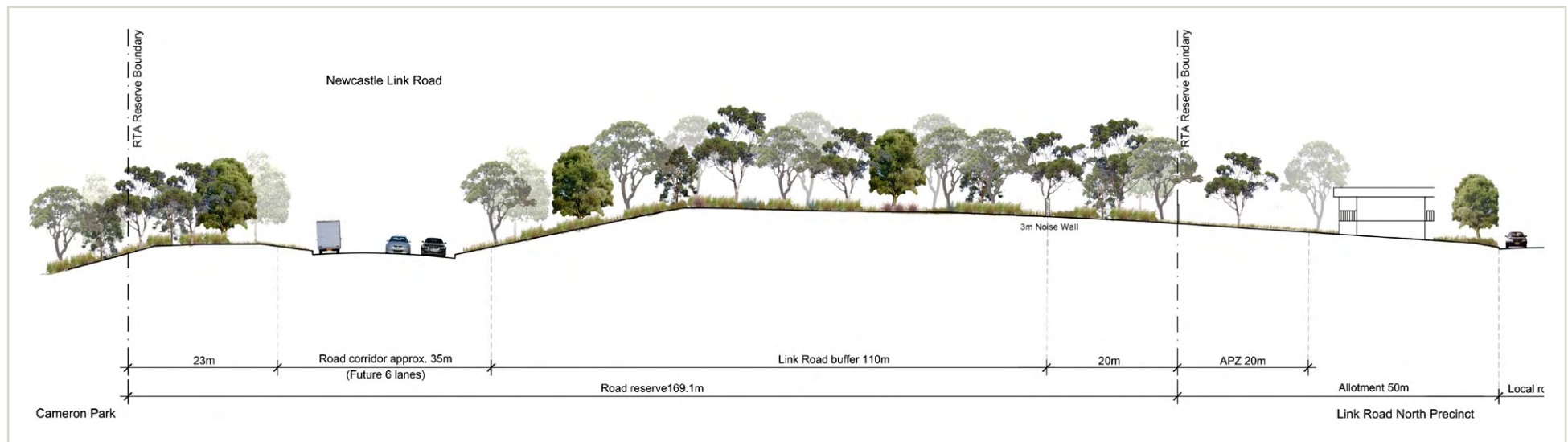
Figure B.1.20. Newcastle Link Road - Cameron Park to Link Road North (Section A-A)
