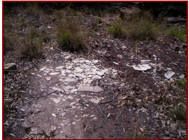
Photo 72 – Fibro fragments on side of track
