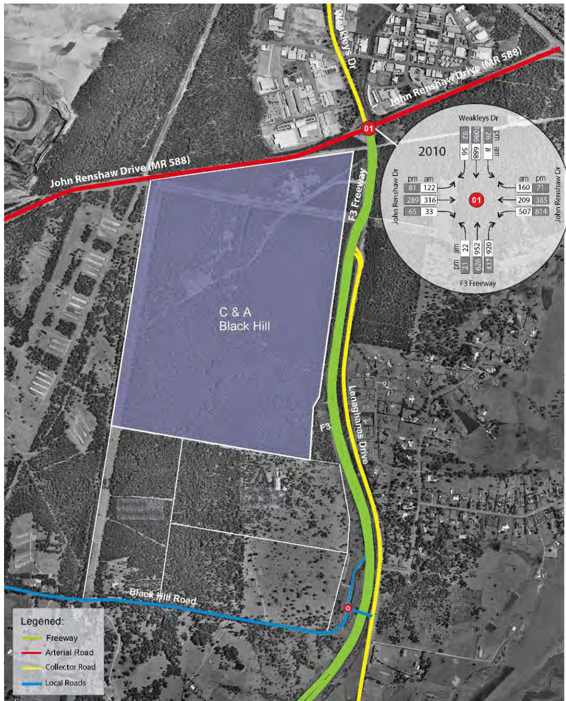
Figure 2-12 Turning volumes (AM, PM peak) data at F3/John Renshaw Drive roundabout in 2010
