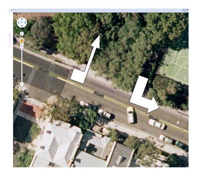
**Figure:** Recommended traffic arrangements if both driveways are used in a one-way system. Note that the turn being made by the car shown turning from Union Street into the current Shore driveway would be illegal, as would be a right-hand turn by a car leaving Shore.
