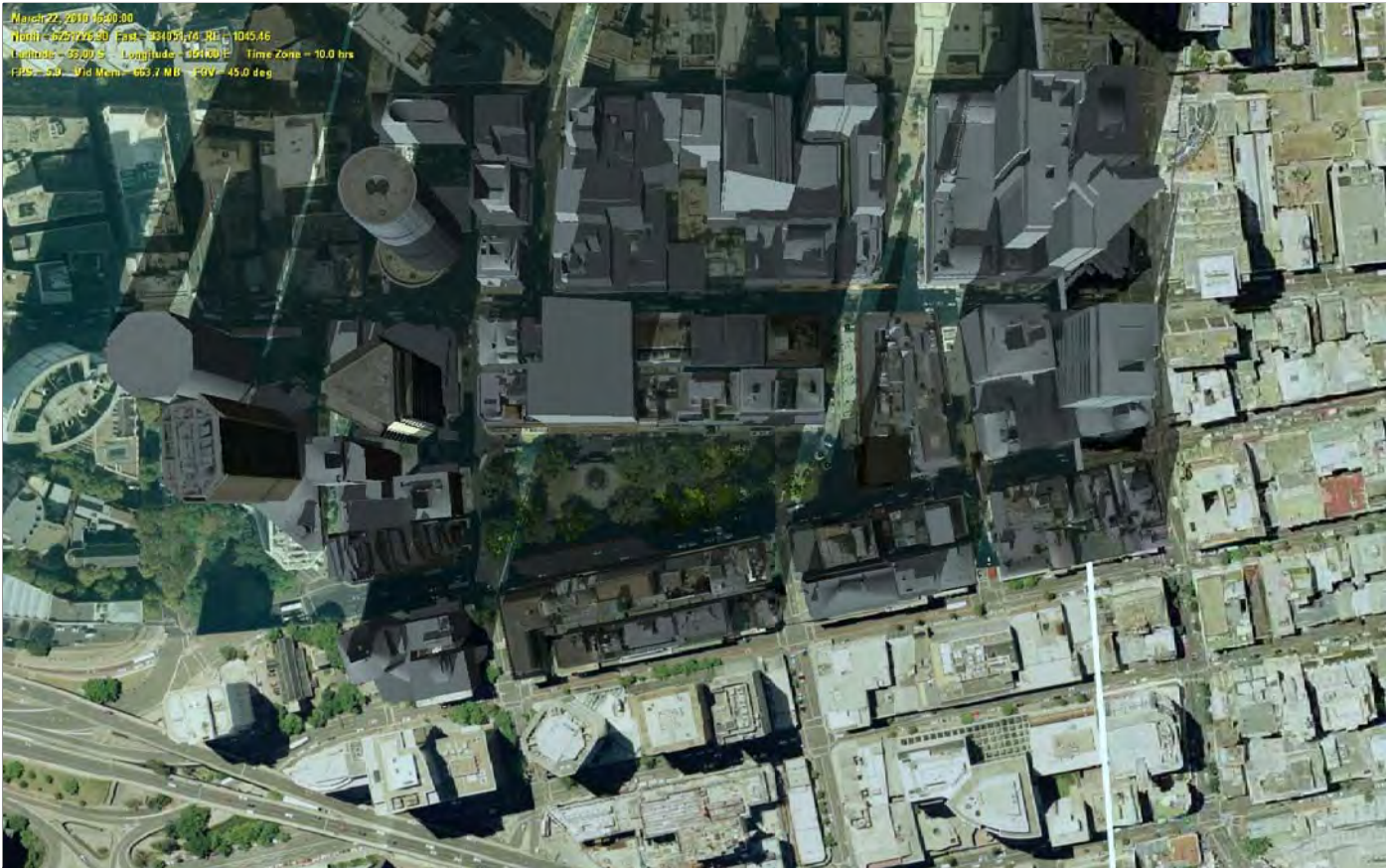
16:00:00 MARCH 22, 2010 SHADOW ANALYSIS FOLLOWING COMPLETION OF PROPOSED CITY ONE PROJECT
