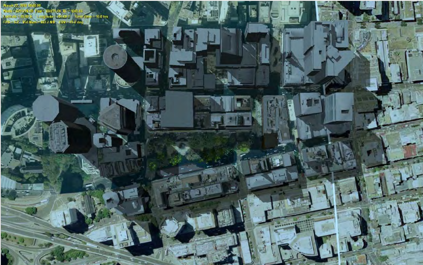
10:00:00 MARCH 22, 2010 SHADOW ANALYSIS FOLLOWING COMPLETION OF PROPOSED CITY ONE PROJECT
