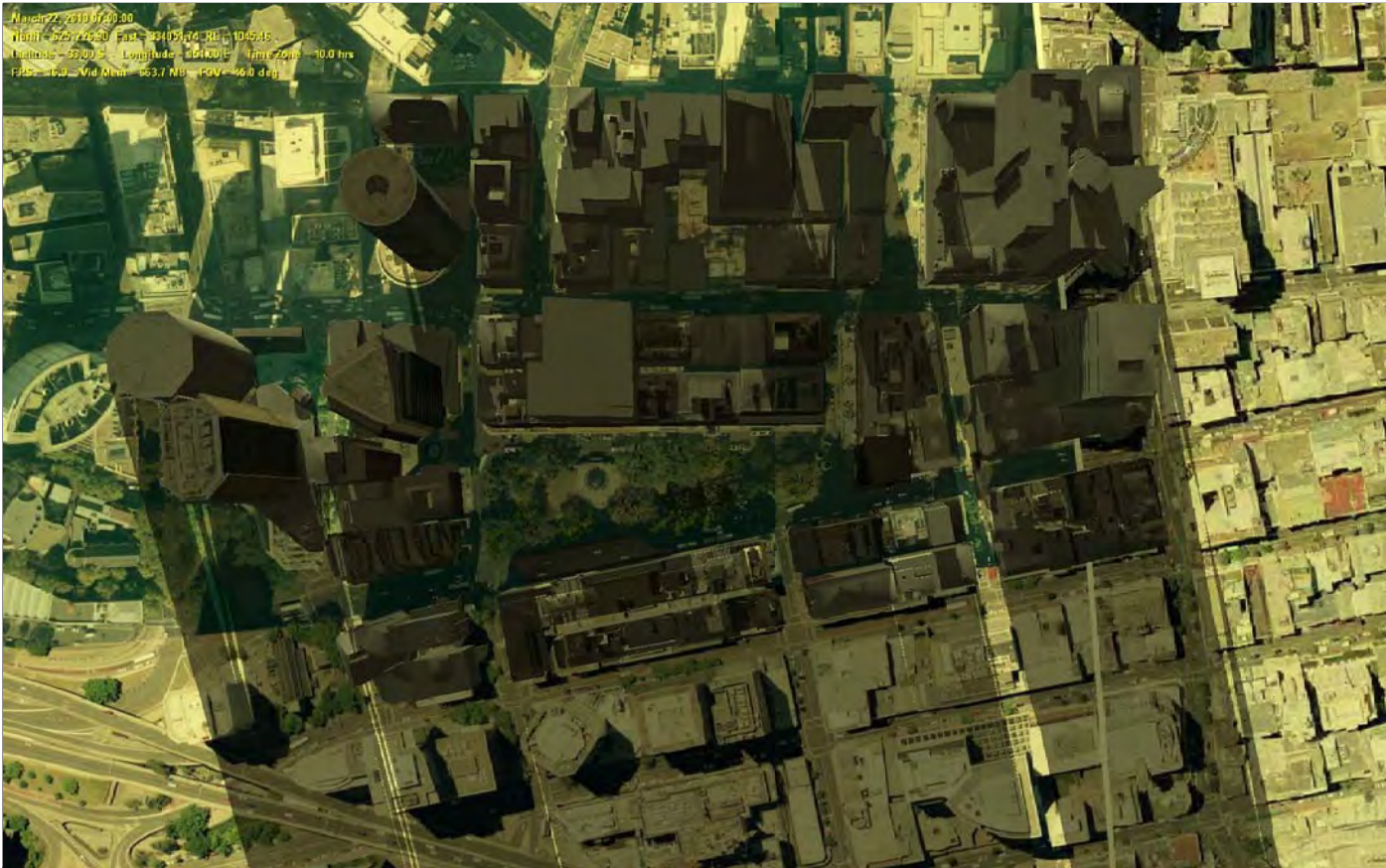
07:00:00 MARCH 22, 2010 SHADOW ANALYSIS FOLLOWING COMPLETION OF PROPOSED CITY ONE PROJECT
