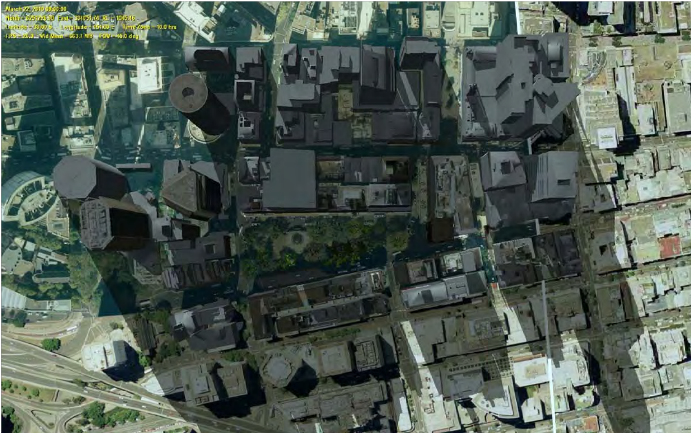
08:00:00 MARCH 22, 2010 SHADOW ANALYSIS FOLLOWING COMPLETION OF PROPOSED CITY ONE PROJECT
