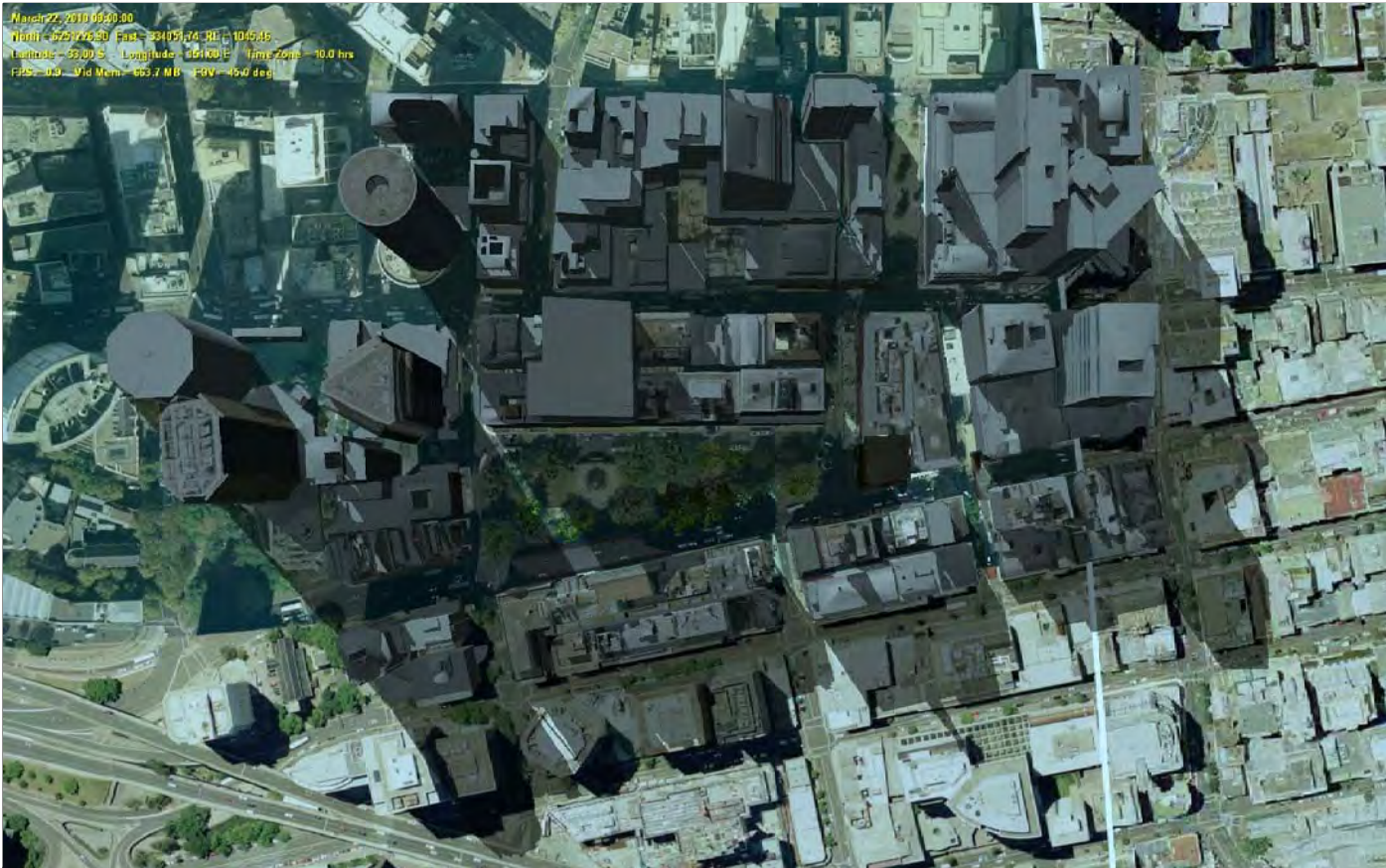
09:00:00 MARCH 22, 2010 SHADOW ANALYSIS FOLLOWING COMPLETION OF PROPOSED CITY ONE PROJECT
