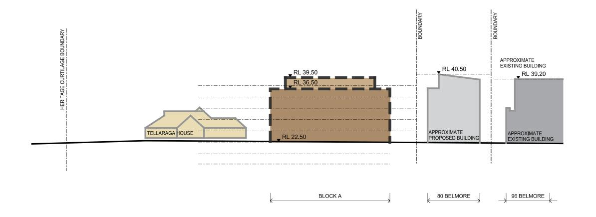
Floor to floor height allows 3m generally. Block F & G are higher, refer drawings.
