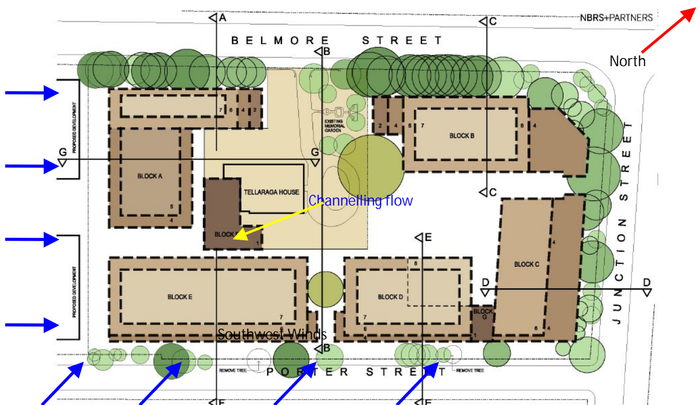
Figure 10: South and Southwest flow and interaction with the development and expected effect.
