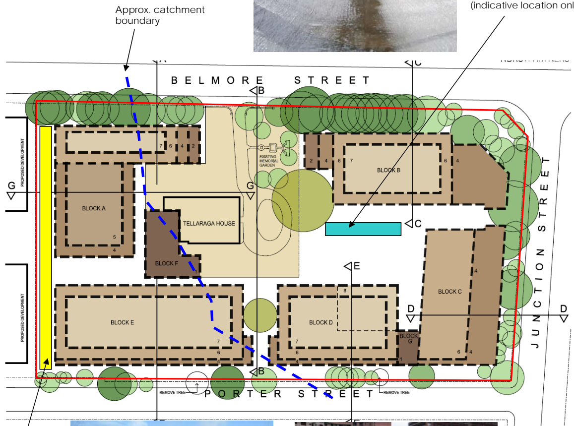
Linear bioretention system to treat runoff from southern part of site, including blocks A, E and F
