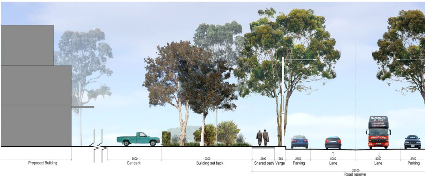
Section AA- 23m wide Road Reserve (Collector road with optional one side Bio-retention swale in verge - alternatively this verge would be landscaped in accordance with the landscape guidelines)
