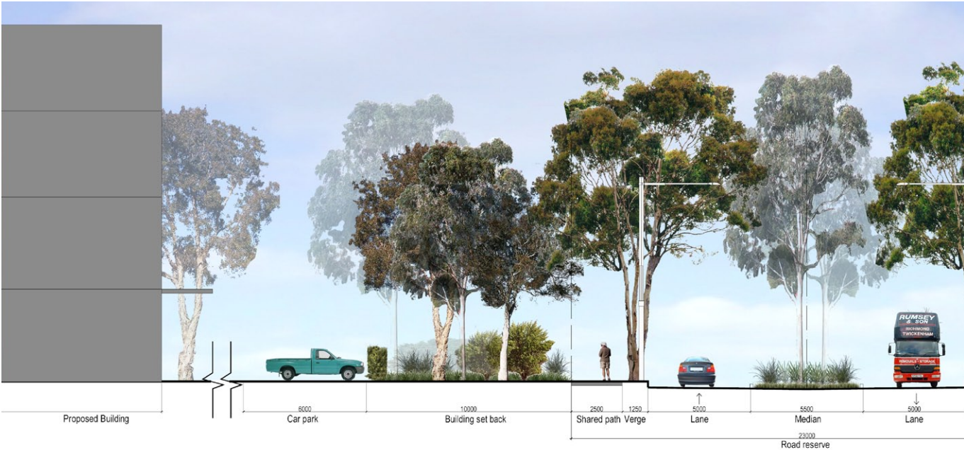
Section BB- 23m wide Road Reserve (Collector road incorporating central median at entry point)
