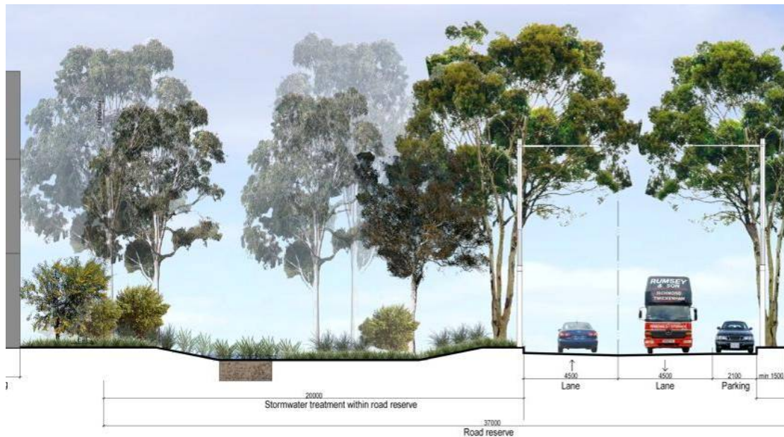
Figure 5 Bioretention systems constructed within road reserve and suitably protected by appropriate landscaping
