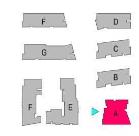
UNITS RECEIVING LESS THAN 2 HRS SOLAR TO LIVING AREAS BETWEEN 9am AND 3pm ON 21/06/11
