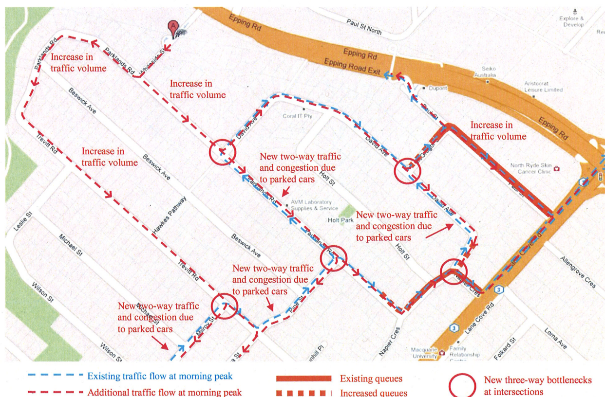
Figure I Flow diagram showing impact of Proposed Whiteside Development on traffic during morning peak
