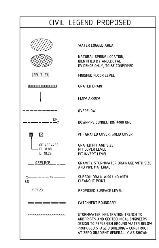
FINAL LOCATION OF PIPES AND PITS TO BE COORDINATED WITH THE LANDSCAPE ARCHITECT AND THE ARBORIST DURING THE PROJECT APPLICATION STAGES OF EACH PROJECT TO ENSURE MINIMUM IMPACT TO EXISTING TREES TO BE
