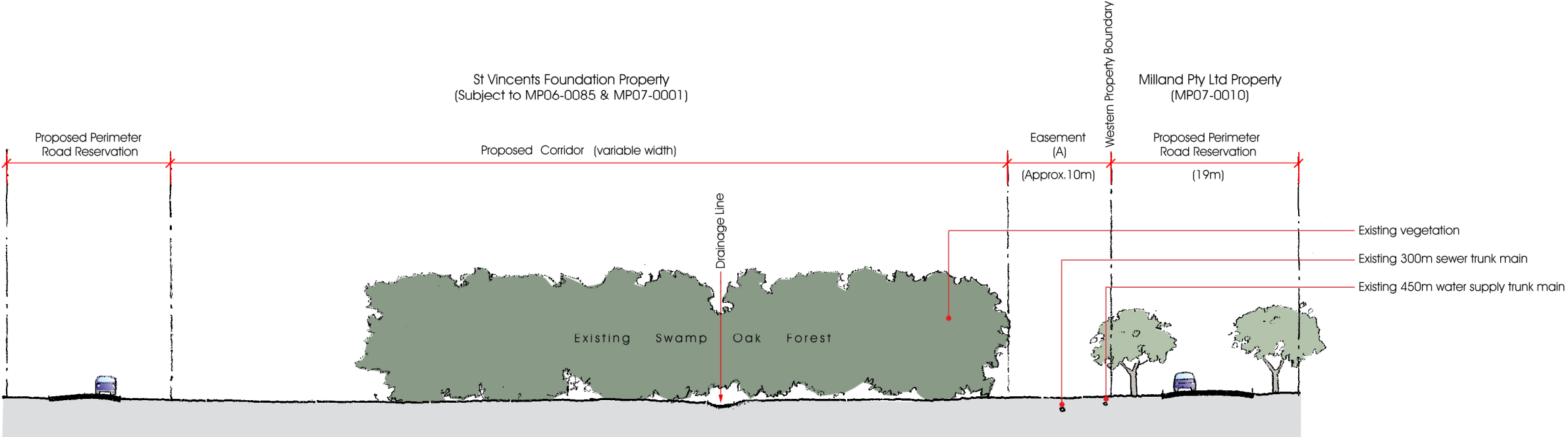
Indicative Cross Section AA Scale 1:500
