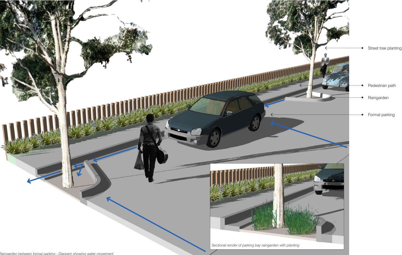
Raingarden between formal parking - Diagram showing water movement
