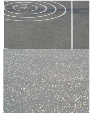
Crusted and graded roof tiles and house bricks
