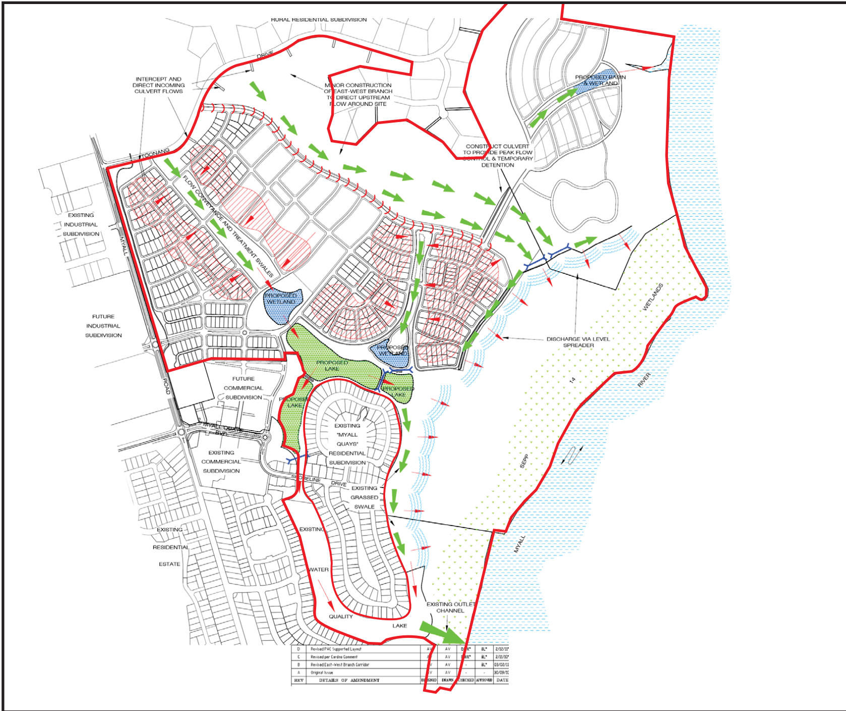
Figure 6.4 Diagrammatic Stormwater Concept Development Plan
