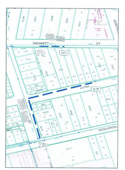
**Wastewater**The existing 225mm sewer shown on the below diagram needs to be amplified to 300mm sewer as **A**to **B** being 217 metres in length and **A** to **C** being 42 metres in length.
