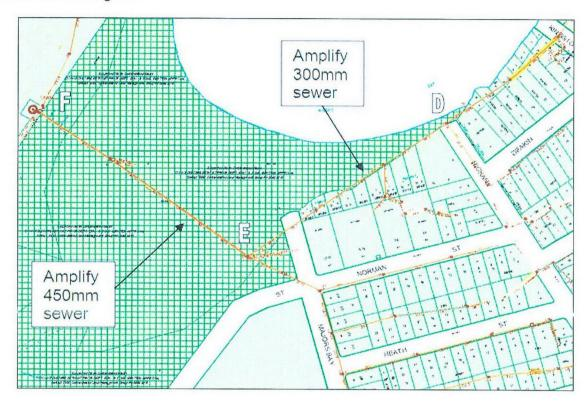
There is no Sydney Water work program for the above amplifications. The SP 090 pump rate is to **remain** as the **current 122 I/s** as these pumps should be increased but cannot due to downstream pipe restrictions.
