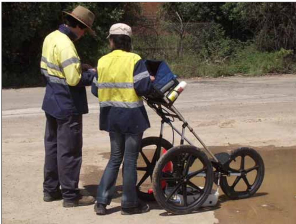
Plate 5: GPR Survey equipment attached to wheel-mounted frame.
