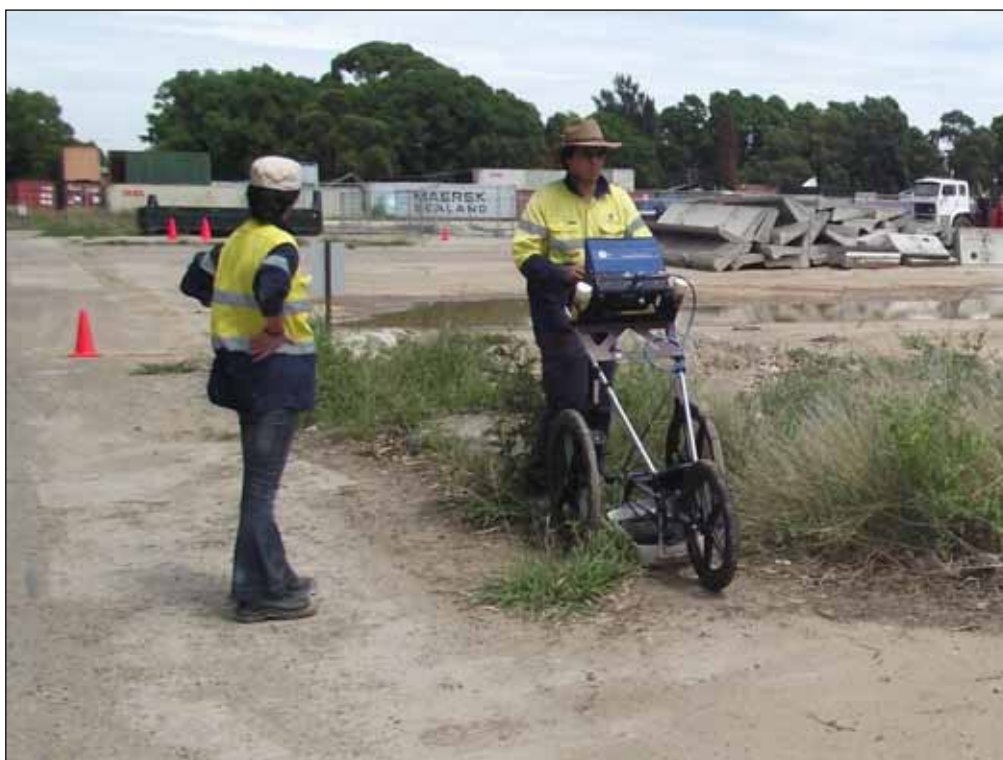
Plate 6: GPR Survey equipment negotiating obstacles, in this case scrub vegetation.
