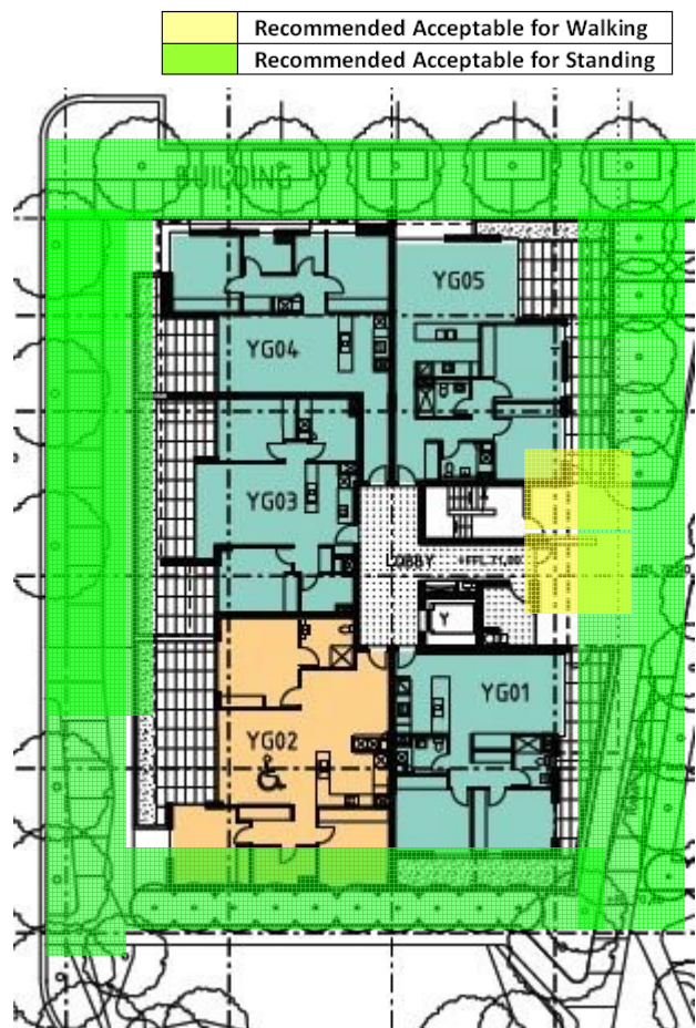
Figure 8: Schematic plan view of the proposed Building Y with the recommended wind criteria overlaid on adjacent ground level areas.
