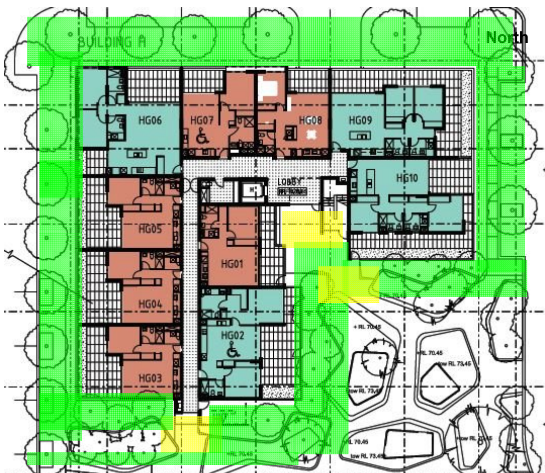
Figure 6: Schematic plan view of the proposed Building H with the recommended wind criteria overlaid on adjacent ground level areas.
