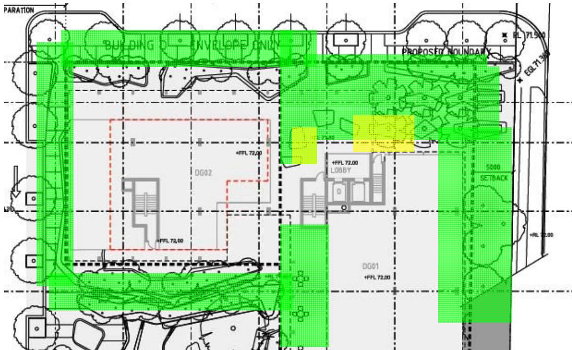
Figure 11: Schematic plan view of the proposed Building D with the recommended wind criteria overlaid on adjacent ground level areas.
