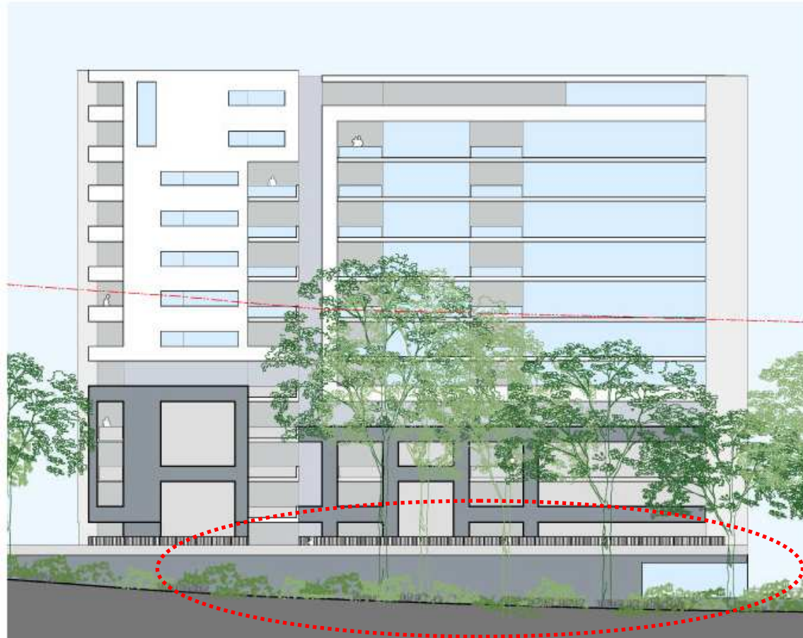
Figure 7: Indicative North Elevation as previously approved As indicated in red, the approved elevation shows the car park level with a blank wall up to 3 metres in height.
